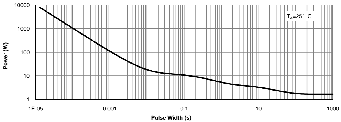
Figure 14: Single Pulse Power Rating Junction-to-Ambient (Note H)
