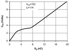
Figure 7: Gate-Charge Characteristics
