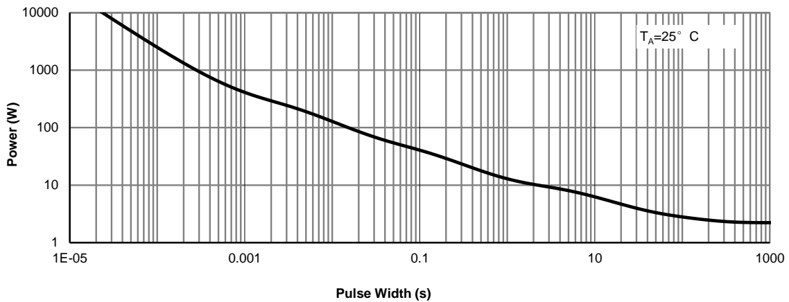
Figure 14: Single Pulse Power Rating Junction-to-Ambient (Note H)
