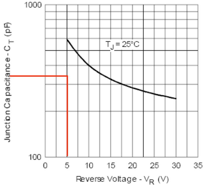
**Figure 5: Junction capacitor of Schottky diode**
