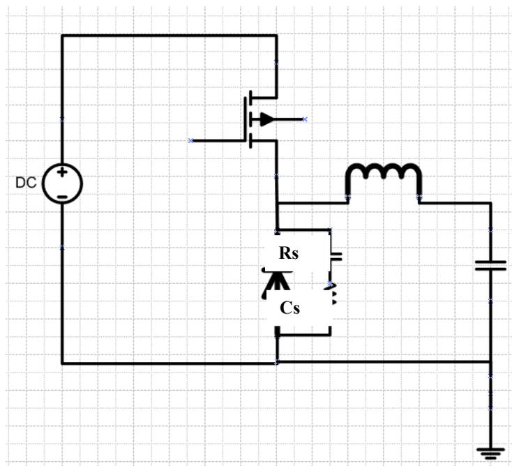
**Figure 1: RC snubber in EZBuck circuit**
