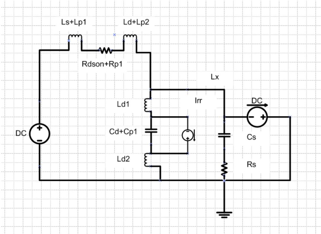
Figure 3: Complete model for PMOS turns on transient of buck converter
