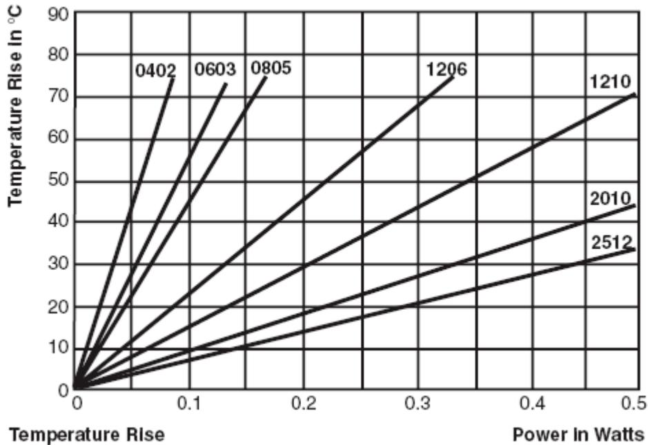
Figure 6: Temperature rise vs. power dissipation
