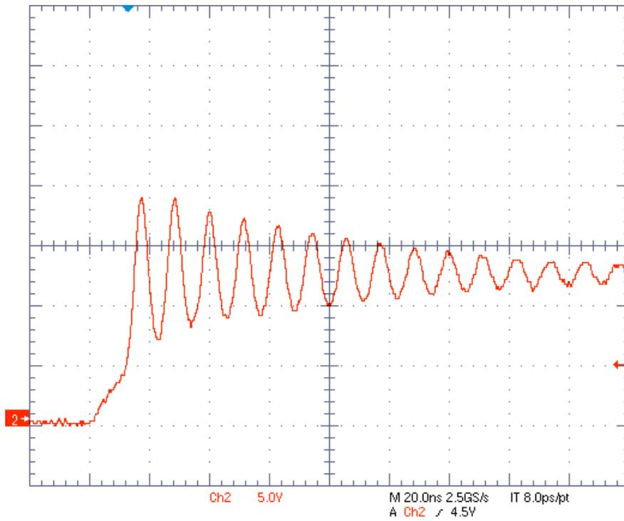
Figure 4: The voltage of LX during PMOS turns on transition
