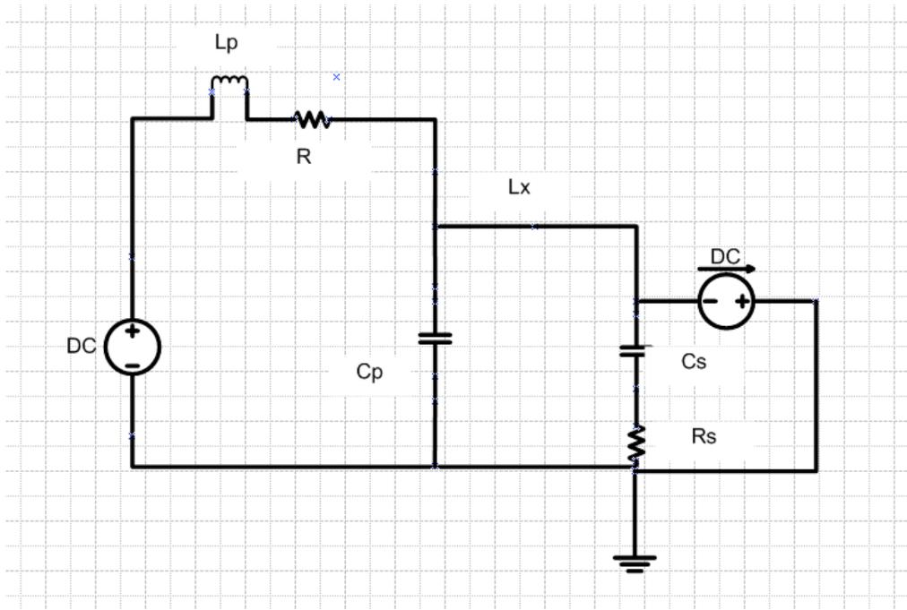
**Figure 2: Over simplified model for PMOS turns on transient of buck converter**
