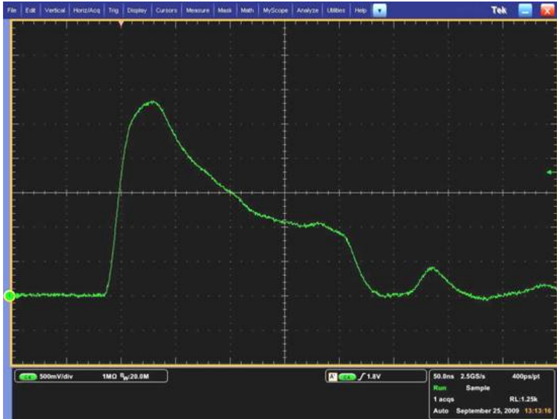
Figure 6. AOZ8802/4 Voltage Clamping Response Waveform at 8kV Contact Discharge. (10X attenuator on scope)
