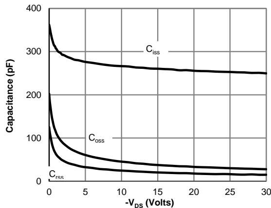
**Figure 8: Capacitance Characteristics**
