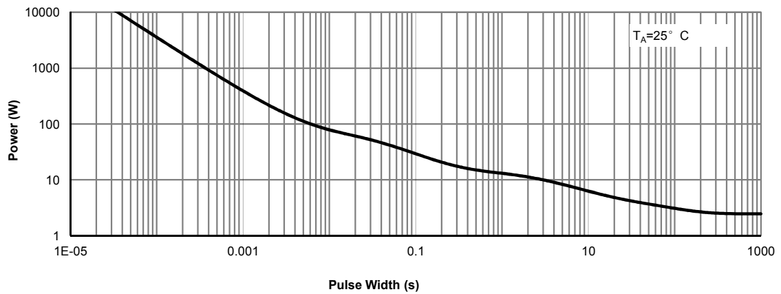
Figure 14: Single Pulse Power Rating Junction-to-Ambient (Note H)
