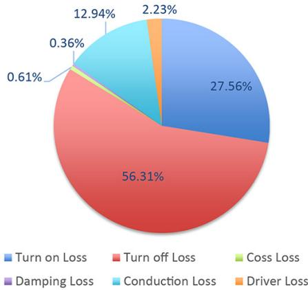
**Power dissipation for one-phase low-side MOSFET AON6500**
