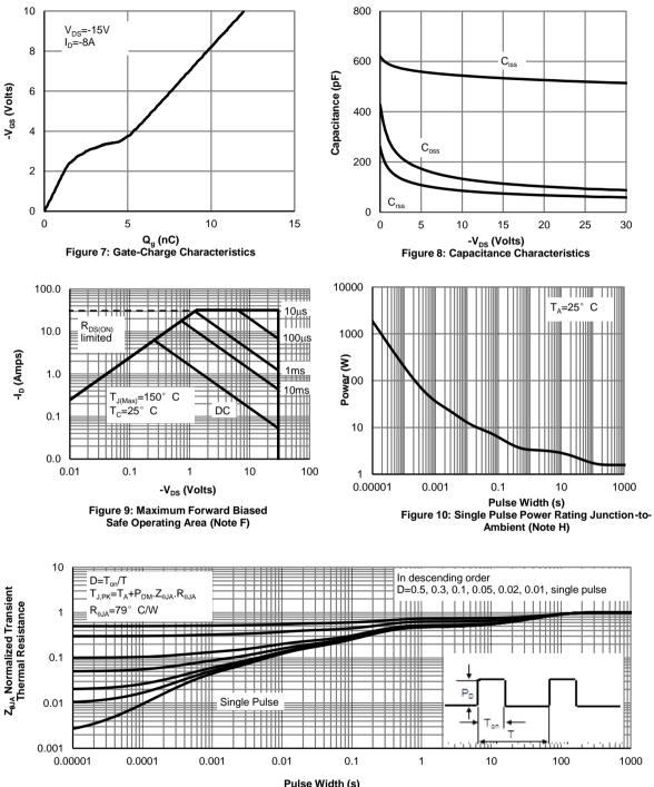
Pulse Width (s) Figure 11: Normalized Maximum Transient Thermal Impedance (Note H)
