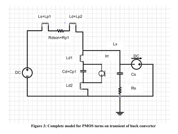
Ls is the source inductor of PMOS and Lp1 is the corresponding parasitic inductor;  $R_{DS(ON)}$  is the  $R_{DS(ON)}$  of PMOS and Rp1 is the trace inductor corresponded; Ld is the drain inductor of PMOS and Lp2 is the corresponding parasitic inductor.
