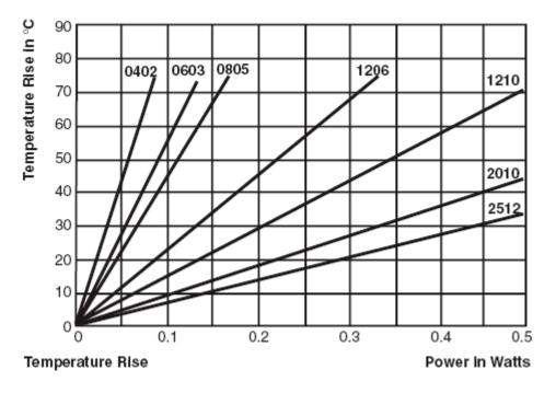
Figure 6: Temperature rise vs. power dissipation
