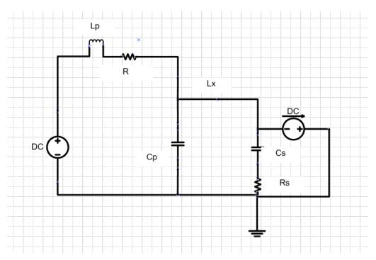
Figure 2: Over simplified model for PMOS turns on transient of buck converter
