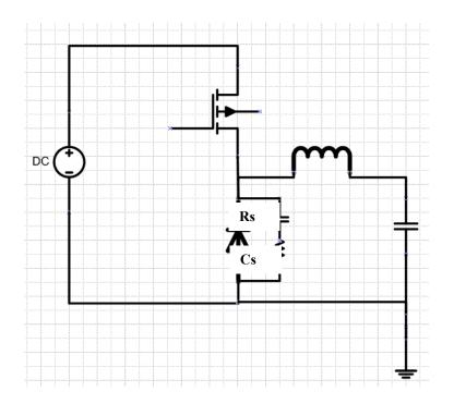
Figure 1: RC snubber in EZBuck circuit
