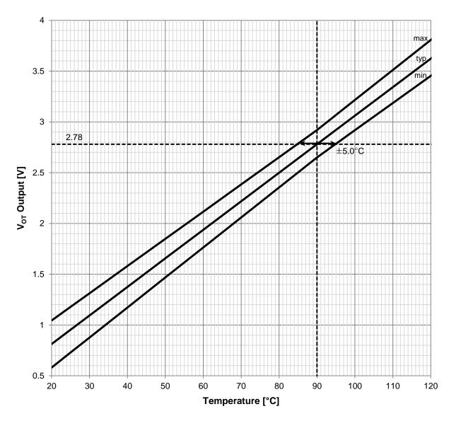
Figure 3. Temperature of LVIC vs.  $V_{\text{OT}}$  Output Characteristics
