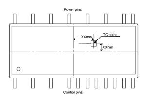
Figure 2. T<sub>C</sub> Measurement Point
