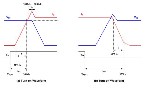
Figure 8. Switching Times Definition
