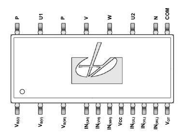
Figure 1. Pin Configuration
