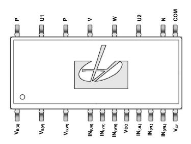
Figure 1. Pin Configuration
