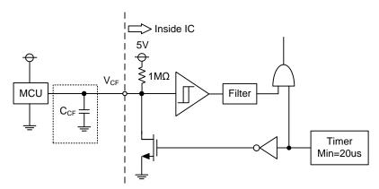
Figure 3. V<sub>CF</sub> Output Circuit
