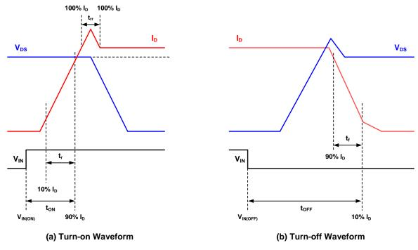
Figure 8. Switching Times Definition
