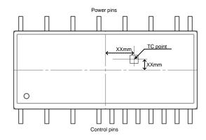
Figure 2. T<sub>C</sub> Measurement Point
