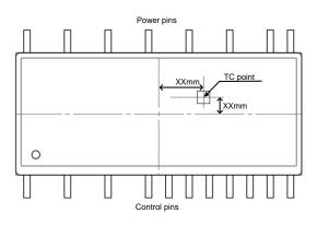
Figure 2. T<sub>c</sub> Measurement Point
