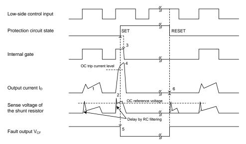
(1) Normal operation: MOSFET turns on and output current.
