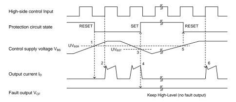
(1) Control supply voltage V<sub>BS</sub> rises. After the voltage reaches under-voltage reset level (UV<sub>BSR</sub>), MOSFETs are turned on by the next ON signal.
