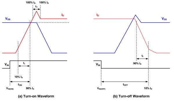
Figure 8. Switching Times Definition
