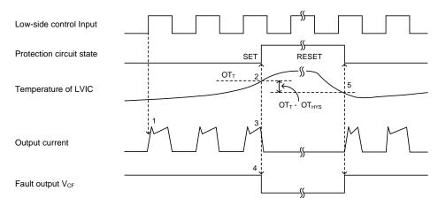
(1) Normal operation: MOSFETs turn on and output current.
