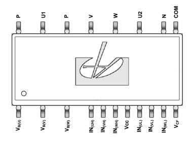
Figure 1. Pin Configuration
