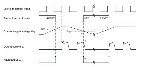
(1) Supply voltage V<sub>CC</sub> becomes higher than under-voltage reset level (UV<sub>CCR</sub>), and MOSFETs are turned on by the next ON signal.
