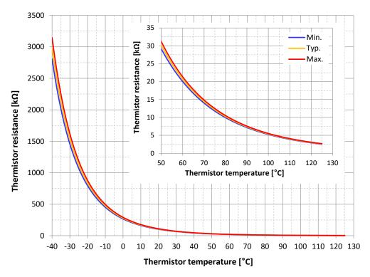
Figure 3. Thermistor Resistance vs. Temperature Curve
