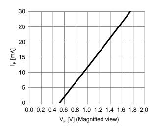
Figure 2. Built-in Bootstrap Diode V<sub>F</sub>-I<sub>F</sub> Characteristic (T<sub>C</sub>=25°C)
