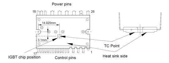
Figure 1. T<sub>C</sub> Measurement Point
