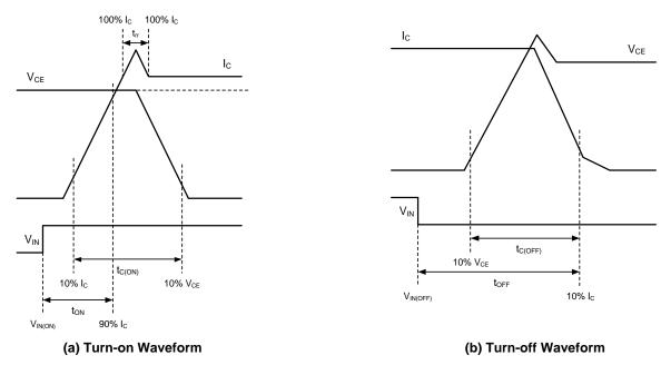
Figure 10. Switching Times Definition
