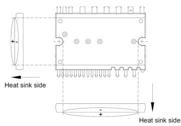
**Figure 5. Flatness Measurement Position**
