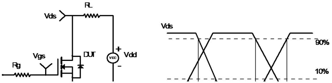
**Unclamped Inductive Switching (UIS) Test Circuit & Waveforms**
