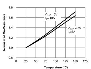
Figure 4: On-Resistance vs. Junction Temperature
