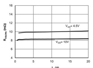
$\label{eq:ldot} {\rm I_D}\left({\rm A}\right)$  Figure 3: On-Resistance vs. Drain Current and Gate Voltage
