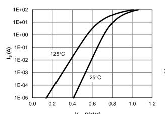
V<sub>SD</sub> (Volts) Figure 6: Body-Diode Characteristics
