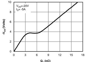
${\bf Q_g}$  (nC) Figure 18: Gate-Charge Characteristics
