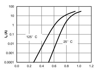
V<sub>SD</sub> (Volts) Figure 6: Body-Diode Characteristics
