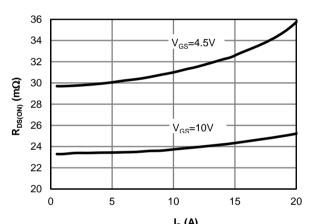
${\rm I_D}\left({\rm A}\right)$  Figure 3: On-Resistance vs. Drain Current and Gate Voltage
