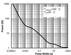
Figure 21: Single Pulse Power Rating Junction-to-Ambient (Note E)
