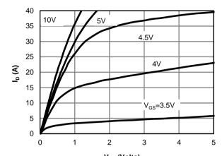
$V_{DS}$  (Volts) Fig 1: On-Region Characteristics
