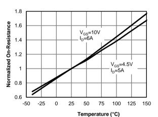
Figure 4: On-Resistance vs. Junction Temperature
