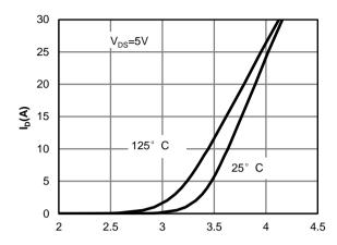
V<sub>GS</sub>(Volts) Figure 2: Transfer Characteristics
