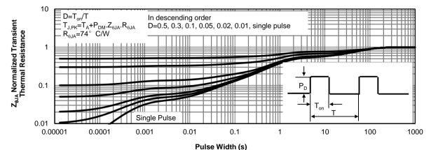
Figure 22: Normalized Maximum Transient Thermal Impedance
