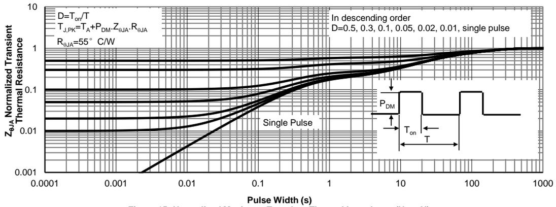
Figure 15: Normalized Maximum Transient Thermal Impedance (Note H)
