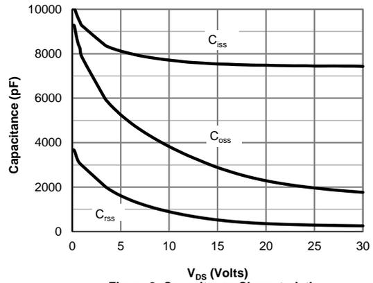
**Figure 8: Capacitance Characteristics**
