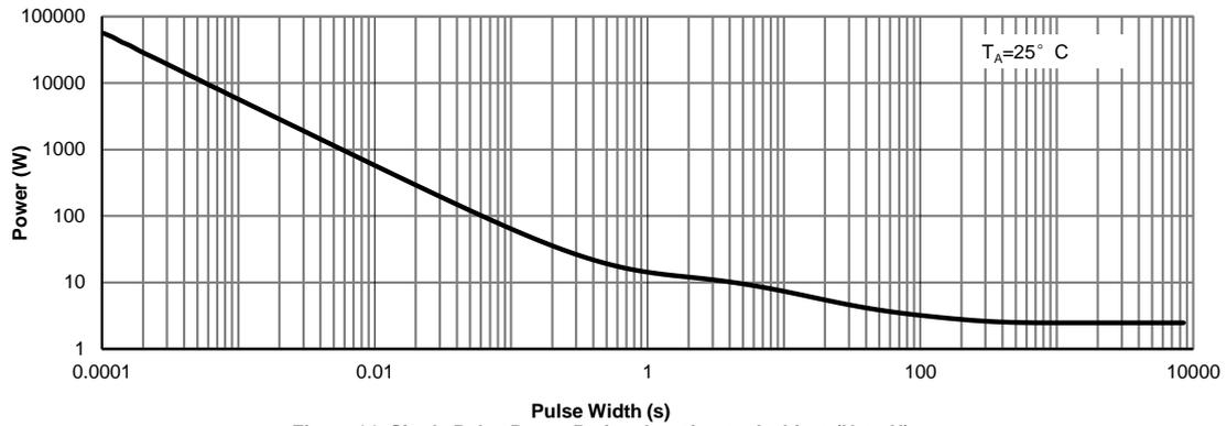
Figure 14: Single Pulse Power Rating Junction-to-Ambient (Note H)
