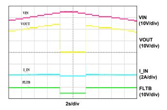
Figure 9. Over Voltage Protection (Option -01)
