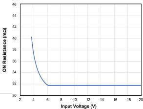
Figure 20. ON Resistance vs. VIN (I<sub>VOUT</sub>=1A)
