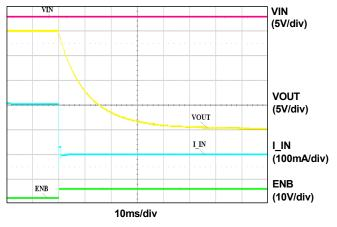
Figure 7. Shutdown (VIN=20V)
