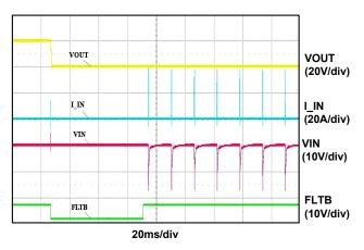
Figure 12. Short Circuit Protection (C<sub>SS</sub>=1nF, No Load, Option -02)
