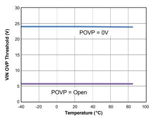
Figure 18. VIN OVP vs. Temperature (I<sub>VOUT</sub>=1A)
