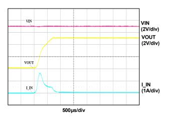
Figure 5. Soft Start Ramp (VIN=5V)
