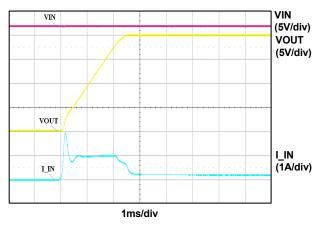
Figure 6. Soft Start Ramp (VIN=20V)
