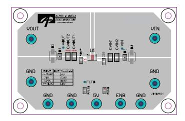
Figure 21. AOZ1324DI Evaluation Board Layout
