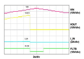
Figure 10. Over Voltage Protection (Option -02)
