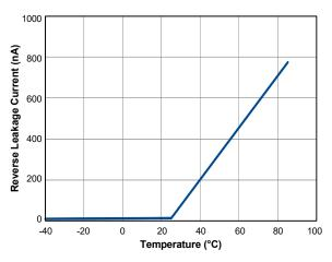
Figure 17. Reverse Leakage Current vs. Temperature
