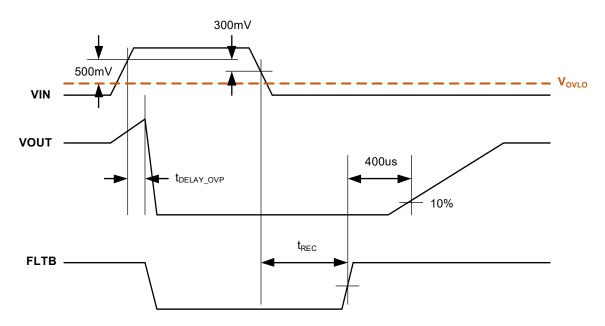
Figure 2. OVP Delay and Recovery Time (AOZ1324DI-01)
