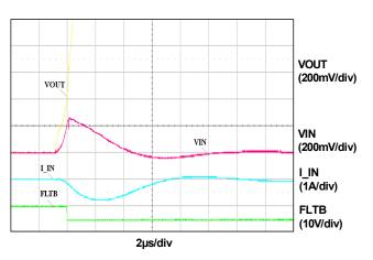
Figure 8. Reverse Current Blocking (VIN=5V)
