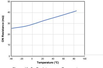
Figure 19. On Resistance vs. Temperature
