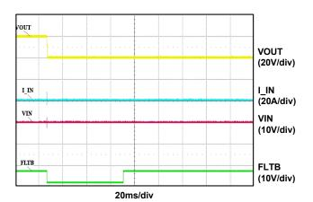
Figure 11. Short Circuit Protection (C<sub>SS</sub>= 1nF, No Load, Option -01)
