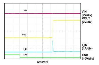
Figure 3. Soft Start Delay Times (VIN=5V)
