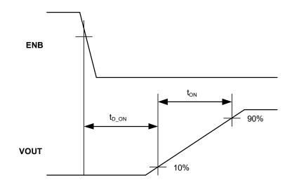
Figure 1. Turn-on Delay and Turn-on Time
