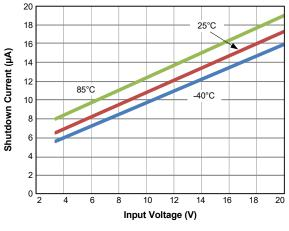
Figure 16. Shutdown Current vs. Input Voltage
