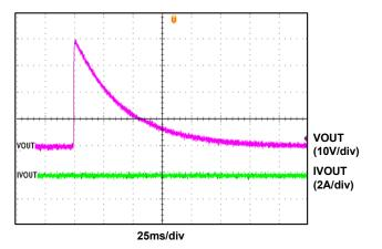
Figure 13. IEC61000-4-5: 40V Surge Voltage without Device
