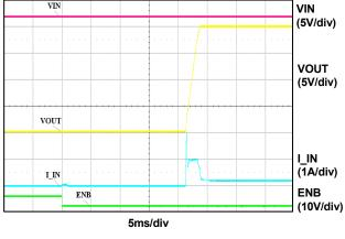
Figure 4. Soft Start Delay Times (VIN=20V)
