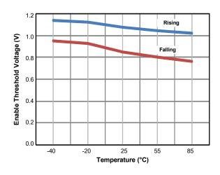
Figure 19. FON Threshold vs. Temperature
