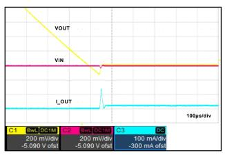
Figure 11. Recovery from Reverse Current Blocking
