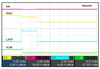
Figure 12. Over Current Protection (Latch-off)
