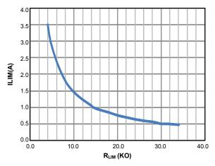
Figure 23. Current Limit vs. R<sub>LIM</sub>
