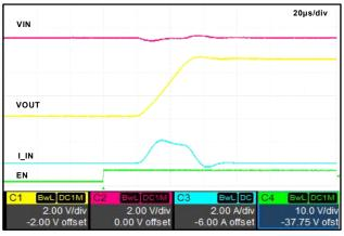
Figure 8. Fast Start Up (FON=5V, No Load)
