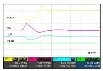
Figure 10. Reverse Current Blocking (VOUT shorted to 20V)
