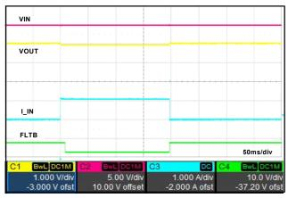
Figure 13. Short Duration Over Current (R<sub>LIM</sub>=14.3K) (Latch-off)
