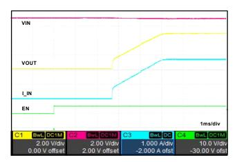
Figure 1. Soft Start (LOAD = 1.9Ω)
