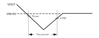
Figure 3. Fast Recovery from RCB
