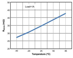
Figure 15. R<sub>DSON</sub> vs. Temperature
