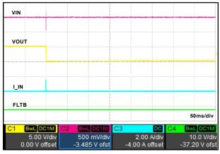
Figure 14. Short Circuit Protection (Latch-off)
