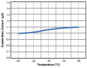
Figure 18. EN Bias Current vs. Temperature
