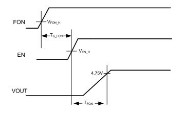
Figure 2. Fast Turn-on Time (VIN=5V)
