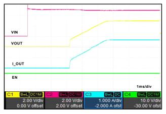
Figure 3. Soft Start by Toggling VIN (LOAD =  $1.9\Omega$ )
