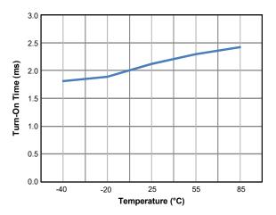
Figure 24. Turn-On Time (TON) vs. Temperature
