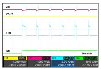
Figure 9. Starting Up into Shorted Output
