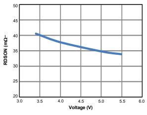
Figure 16. RDSON vs. Input Voltage
