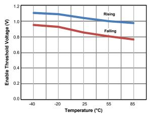
Figure 17. EN Threshold vs. Temperature
