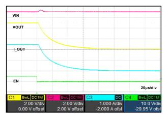
Figure 2. Shutdown by EN (LOAD =  $1.9\Omega$ )
