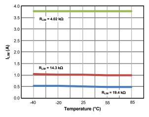
Figure 22. Current Limit Threshold vs. Temperature
