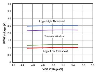
Figure 10. PWM Threshold vs. VCC Voltage
