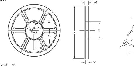
TAPE SIZE REEL SIZE М Ν W W1 Н К S G R V ø330.0 ±2.0 ø79.0 ±1.0 ø13.0 ±0.5 10.5 ±0.2 2.0 ±0.5 12.4 17.0 \_\_\_ \_\_\_\_ \_\_\_\_ 12 mm Ø330 +2.0 -0.0 +2.6 -1.2
