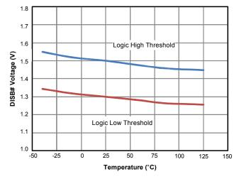
Figure 9. DISB# Thereshold vs. Temperature
