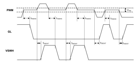
Figure 2. PWM Tri-State Hold Off and Exit Timing Diagram
