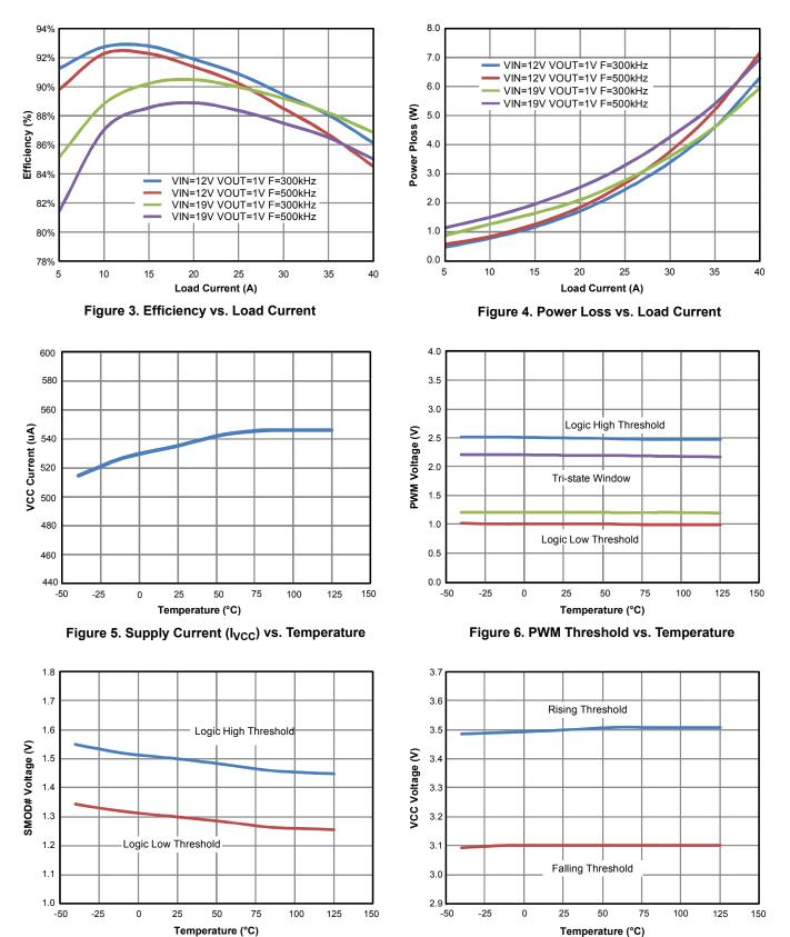
Figure 7. SMOD# Threshold vs. Temperature
