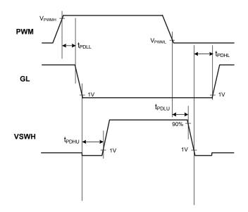
Figure 1. PWM Logic Input Timing Diagram
