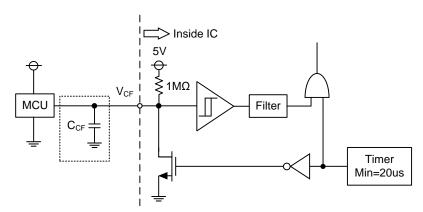
Figure 3. V<sub>CF</sub> Output Circuit
