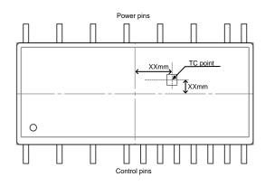
Figure 2. Tc Measurement Point
