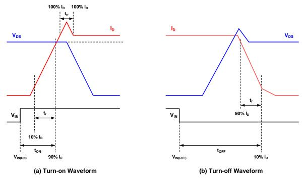
Figure 8. Switching Times Definition
