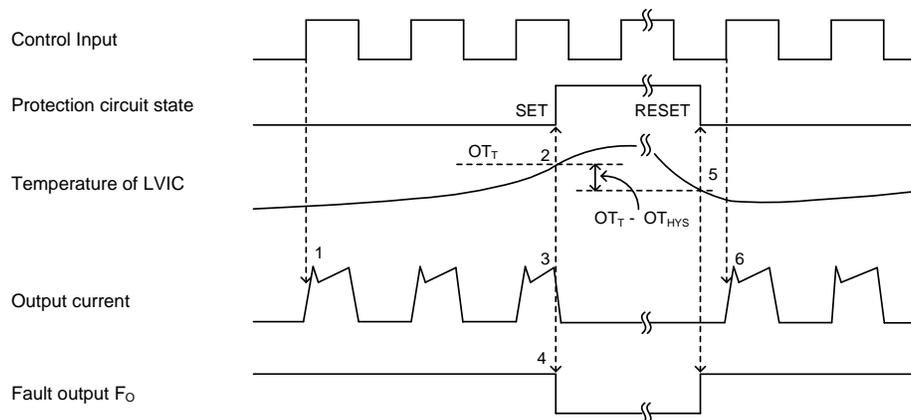
**Figure 10. Over-Temperature Protection (Low-side, Detecting LVIC Temperature)**
