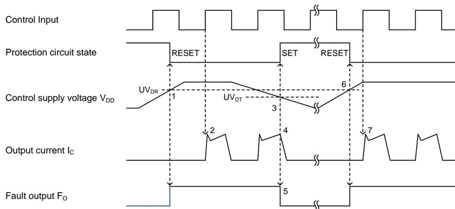
**Figure 8. Under-Voltage Protection (Low-side, UV<sub>D</sub>)**
