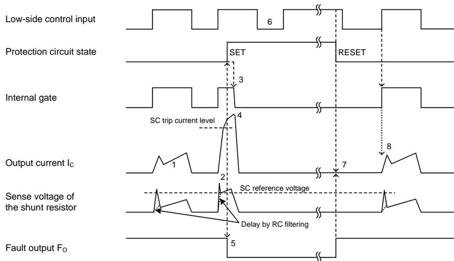
**Figure 7. Short-Circuit Protection
