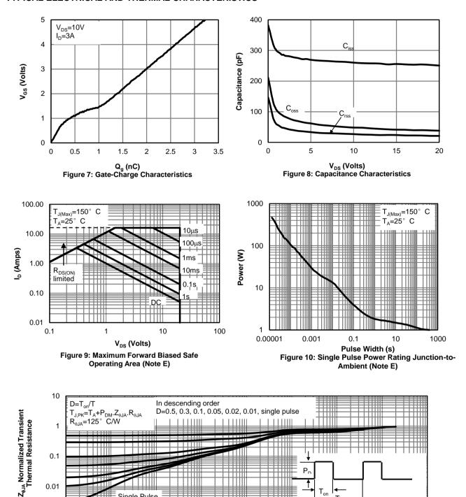
Pulse Width (s) Figure 11: Normalized Maximum Transient Thermal Impedance (Note E)
