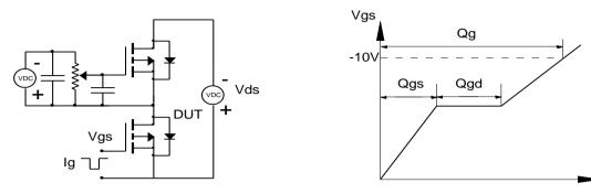
Resistive Switching Test Circuit & Waveforms
