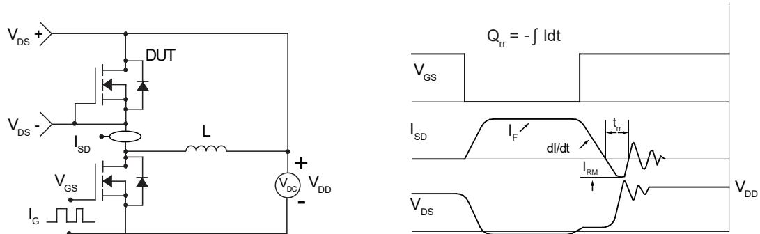
Figure 21. Diode Recovery Test Circuits and Waveforms
