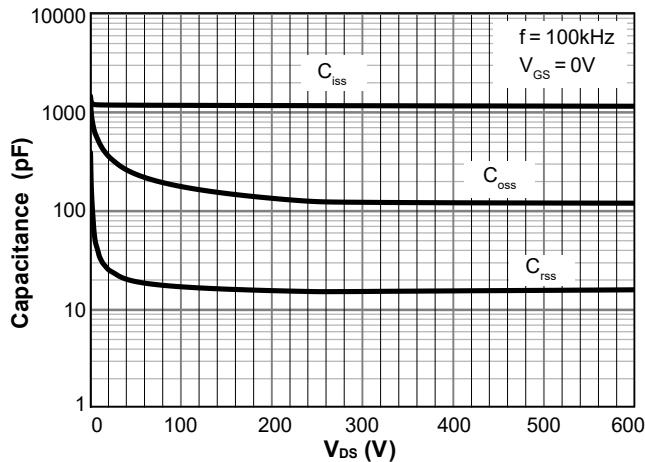
Figure 10. Capacitance Characteristics
