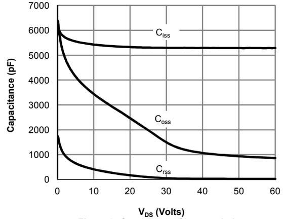
**Figure 8: Capacitance Characteristics**
