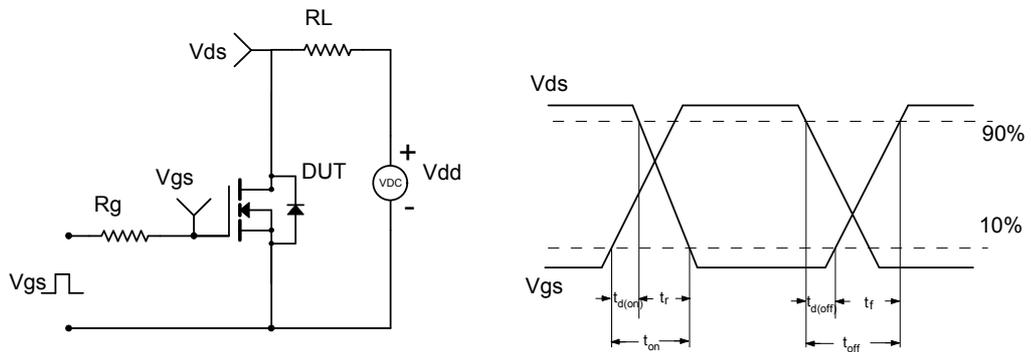
Figure C: Unclamped Inductive Switching (UIS) Test Circuit & Waveforms
