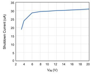
Figure 4. Shutdown Current vs. VIN
