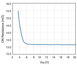
Figure 5. On Resistance vs. VIN
