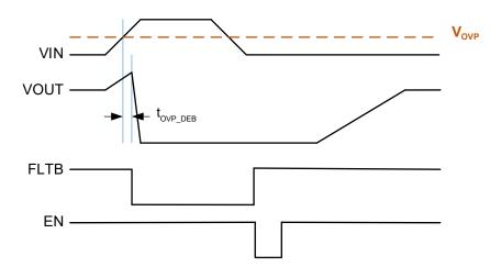
Figure 2. Over-Voltage Protection
