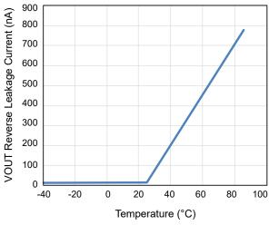
Figure 7. VOUT Reverse Current Leakage vs. Temperature
