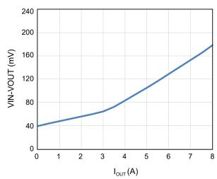
Figure 8. Ideal Diode Regulation Voltage vs.  $I_{OUT}$
