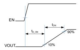
Figure 1. Turn-on Delay and Turn-on Time
