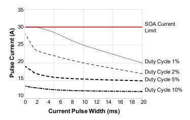
Figure 11. AOZ13289DI-01 Sinking Switch Pulsed Current vs. Duration for a Given Duty Cycle
