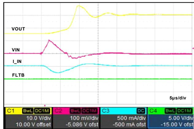
Figure 10. Reverse Current Blocking (VOUT shorted to 20V)
