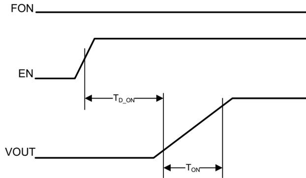
Figure 1. Normal Turn-on Delay and Turn-on Time ( $V_{FON}=0V$ )
