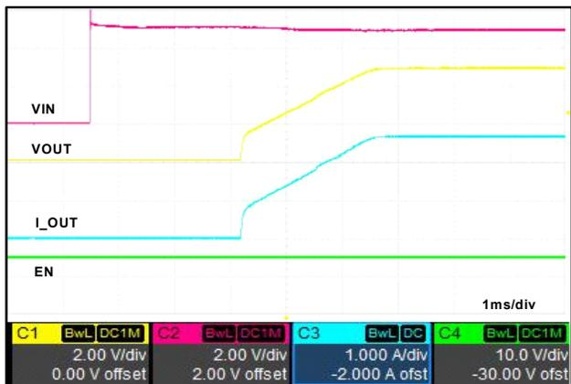
Figure 3. Soft Start by Toggling VIN (LOAD = 1.9Ω)
