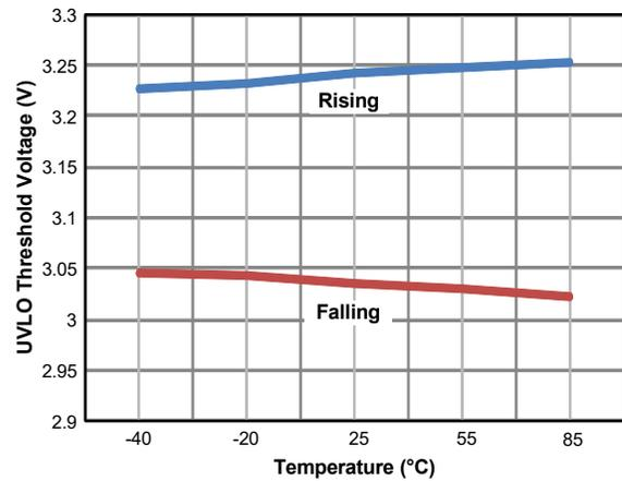
Figure 20. UVLO Threshold vs. Temperature (AOZ1356LI-01, -02)
