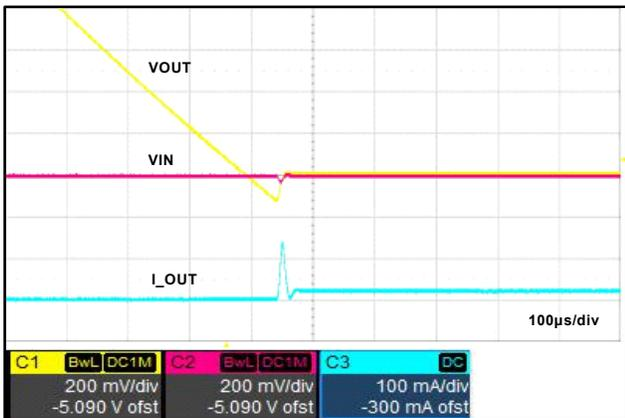
Figure 11. Recovery from Reverse Current Blocking
