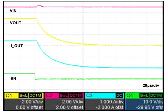
Figure 2. Shutdown by EN (LOAD = 1.9Ω)
