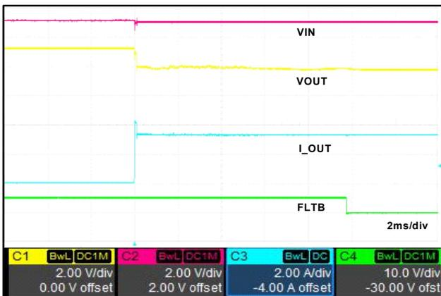
Figure 5. Over Current Protection (LOAD = 1.2Ω Plugged In)
