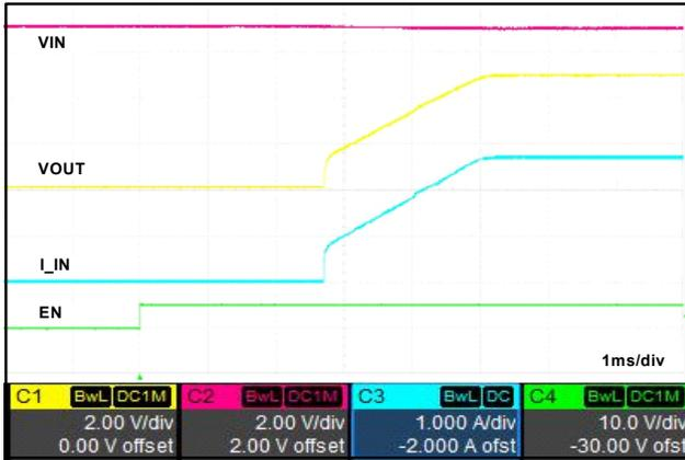
Figure 1. Soft Start (LOAD = 1.9Ω)
