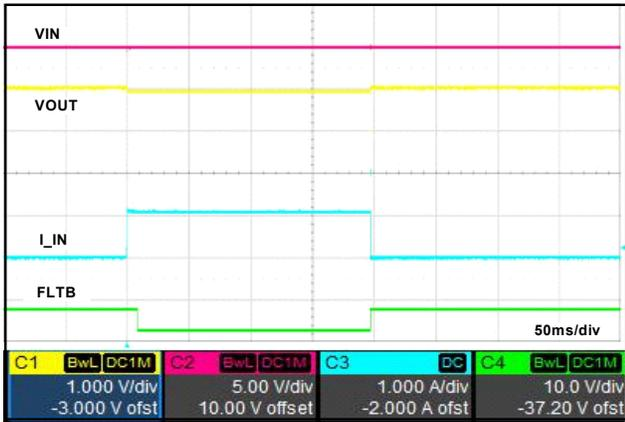
Figure 13. Short Duration Over Current ( $R_{LIM}=14.3\text{K}$ ) (Latch-off)
