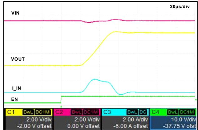
Figure 8. Fast Start Up (FON=5V, No Load)
