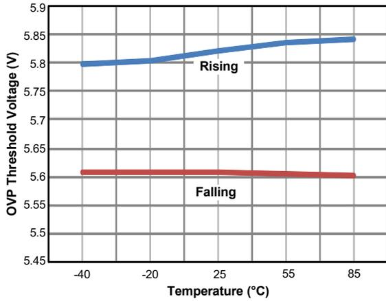
Figure 21. OVP Threshold vs. Temperature (AOZ1356LI-01, -02)
