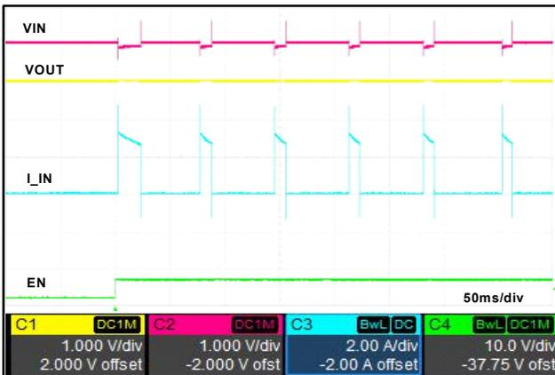
Figure 9. Starting Up into Shorted Output
