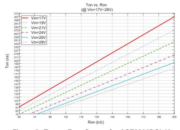
Figure 5. T<sub>ON</sub> vs. R<sub>TON</sub> Curves for AOZ2260DQI-10
