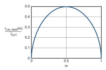
Figure 6. I<sub>CIN</sub> vs. Voltage Conversion Ratio
