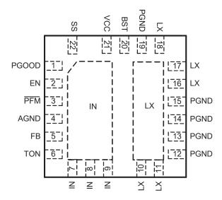
Figure 1. AOZ2260DQI-10 22-Pin 4mmx4mm QFN
