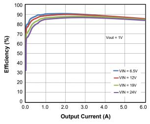
Figure 2. Efficiency vs. Load Current
