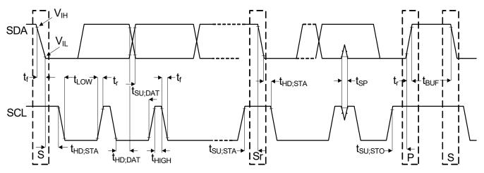
Figure 1. I<sup>2</sup>C Timing Definitions
