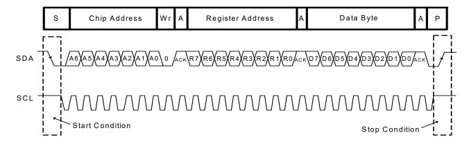
Figure 2. A Complete Write Byte Transfer
