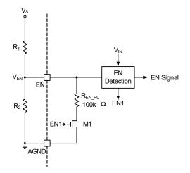
Figure 6. Enable Internal Circuit
