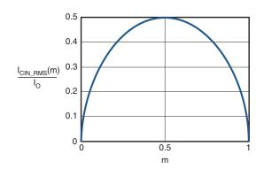
Figure 13. I<sub>CIN</sub> vs. Voltage Conversion Ratio
