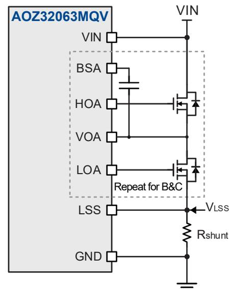
Figure 5. LSS Voltage ( $V_{LSS}$ )
