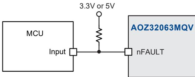
Figure 2. nFAULT Pin Application Circuit
