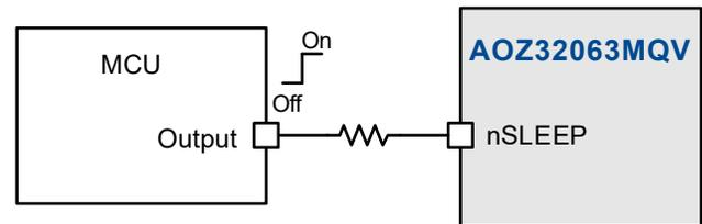
Figure 1. nSLEEP Pin Application Circuit
