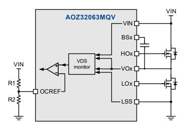
Figure 6. MOSFET VDS Sensing and OCREF Pin Application Circuit
