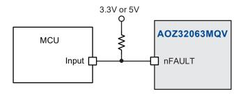
Figure 2. nFAULT Pin Application Circuit
