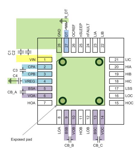
Figure 7. Layout Reference Diagram
