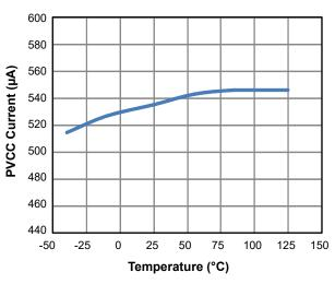
Figure 5. Supply Current ( $I_{VCC}$ ) vs. Temperature
