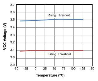
Figure 8. UVLO (VCC) Threshold vs. Temperature
