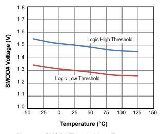
Figure 7. SMOD# Threshold vs. Temperature
