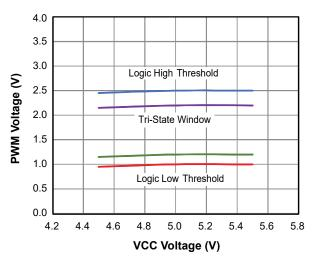
Figure 10. PWM Threshold vs. VCC Voltage
