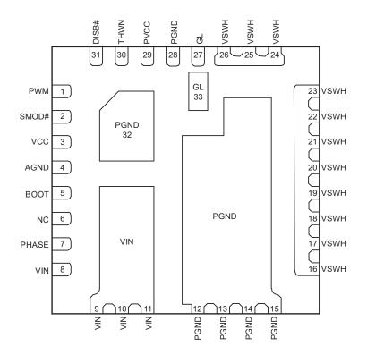
QFN5x5-31L (Top View)
