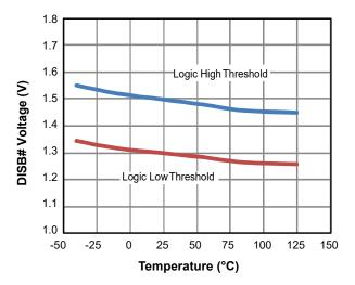
Figure 9. DISB# Threshold vs. Temperature
