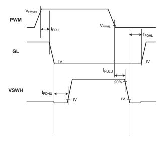
Figure 1. PWM Logic Input Timing Diagram
