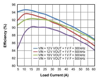
Figure 3. Efficiency vs. Load Current
