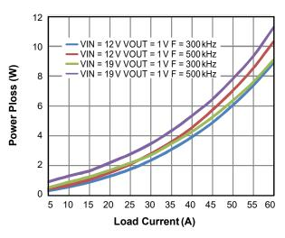
Figure 4. Power Loss vs. Load Current
