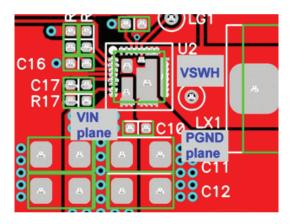
Figure 13. Top Layer of Demo Board, VIN, VSWH and PGND Copper Planes
