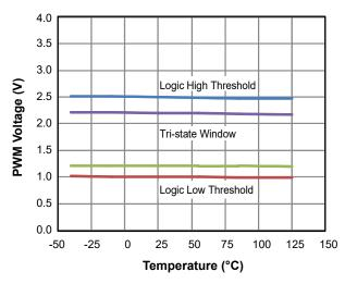
Figure 6. PWM Threshold vs. Temperature
