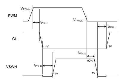
Figure 1. PWM Logic Input Timing Diagram
