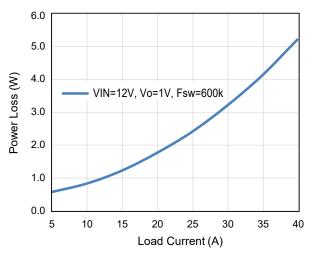
Figure 4. Power Loss vs Load Current
