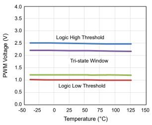
Figure 5. PWM Threshold vs. Temperature
