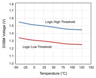
Figure 7. DISB# Threshold vs Temperature
