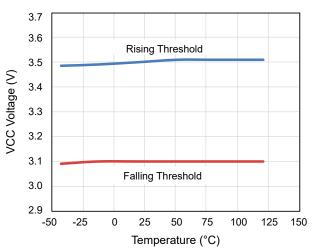
Figure 6. UVLO (VCC) Threshold vs. Temperature
