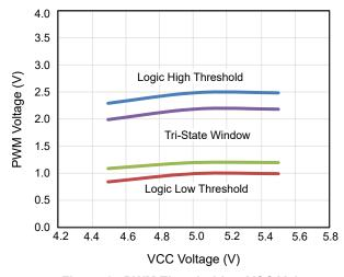
Figure 8. PWM Threshold vs VCC Voltage
