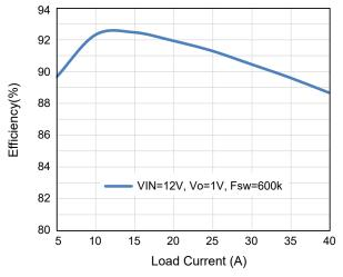
Figure 3. Efficiency vs Load Current
