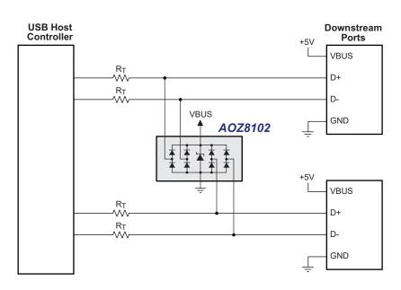
Figure 1. 2 USB High Speed Ports
