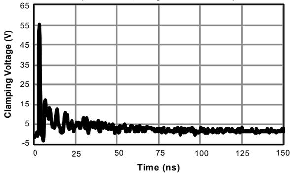
**-8kV ESD Clamping Per IEC 61000-4-2**
