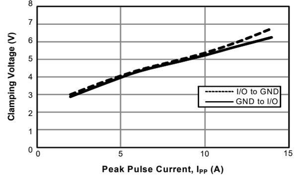
**+8kV ESD Clamping Per IEC61000-4-2**
