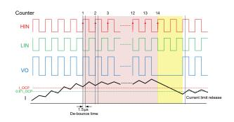
Figure 13. OCP timing diagram
