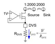
Figure 14. Source/Sink Current Setting
