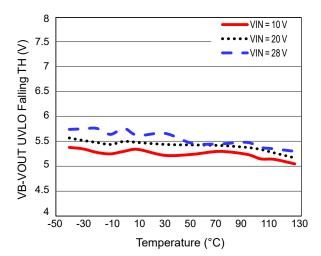
Figure 5. VB-VOUT UVLO Falling Threshold
