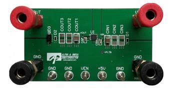
Figure 1. Top View of AOZ13984/87DI EVB
