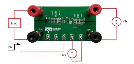
Figure 3. AOZ13984/87DI Evaluation Board Set Up
