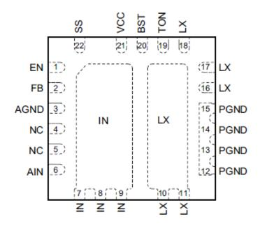
22-Pin 4mm x 4mm QFN (Top View)
