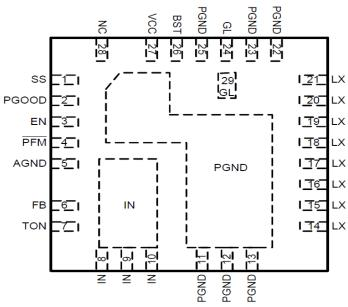
28-Pin 5mm x 5mm QFN (Top View)
